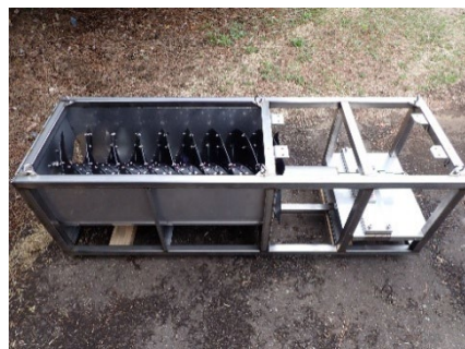
Fig.1 らせん水車 Spiral Water Turbine
